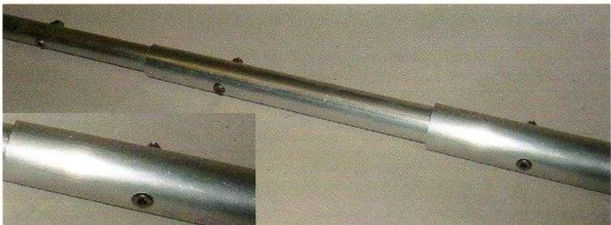
Ansicht Elementübergänge 25/20mm - 20/16mm - 16/12mm / close up view element transitions 25/20mm - 20/16mm - 16/12mm
